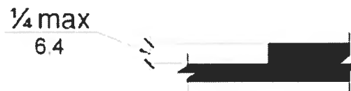
Figure 303.2 Vertical Change in Level
