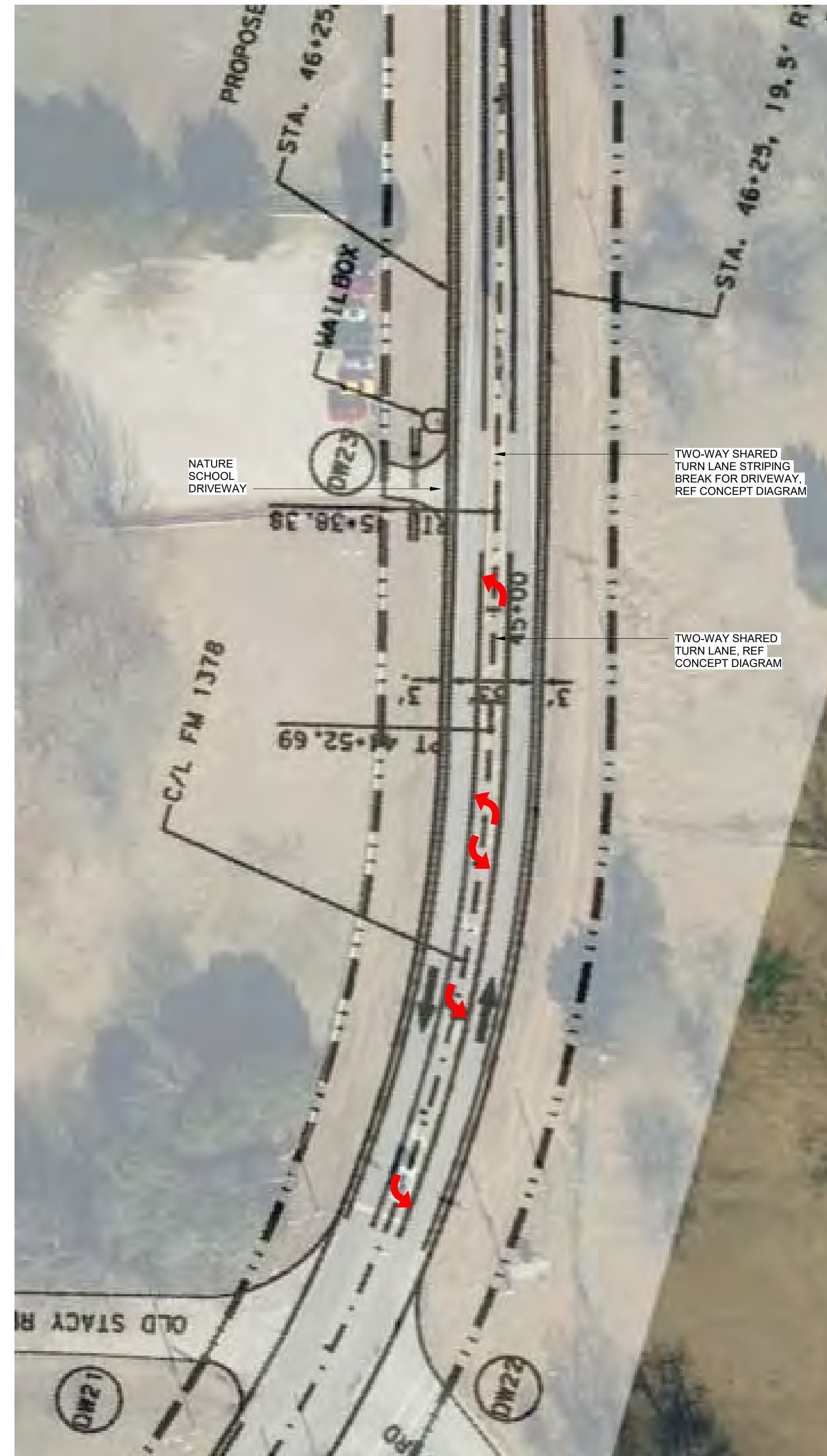
① TXDOT PROPOSED ROADWAY IMPROVEMENTS - TIA STRIPING RECOMMENDATIONS 1/2" = 1'-0"
